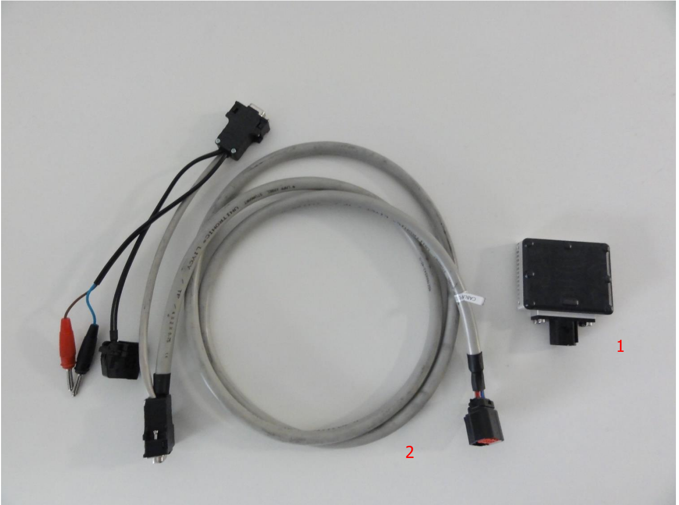
Picture 3: UMRR-8F Type 146 (1) with compatible CABLE-FF0025 (2)
