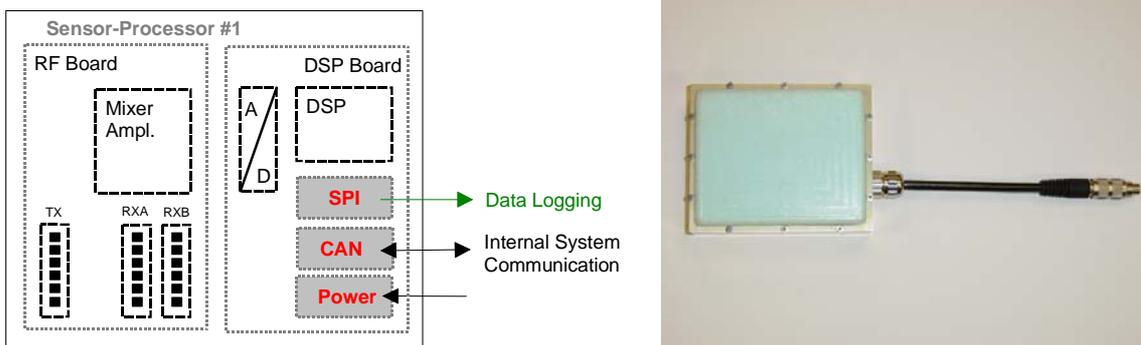
Figure 1: Block Diagram and Photograph of the UMRR Radar Sensor
