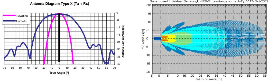
Figure 4: Example Antenna diagram and Dual Sensor configuration on a test car.
