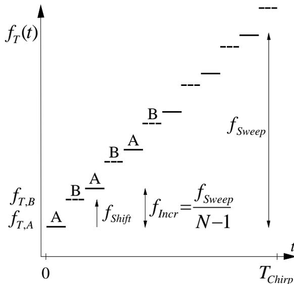
Figure 3: FMSK-2 Transmit Waveform
