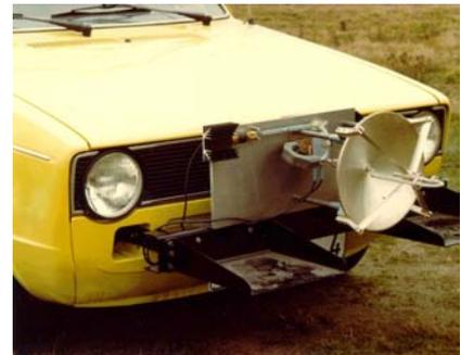
Thus economical and manufacturing conditions in this market are completely different with respect radars for defense applications. One first application for automotive radar sensors was the Adaptive Cruise Control (ACC) function. It was introduced first in passenger cars in 1998 as a comfort feature. (The cruise control systems previously controlled speed only but did not control the distance to the vehicle ahead).
