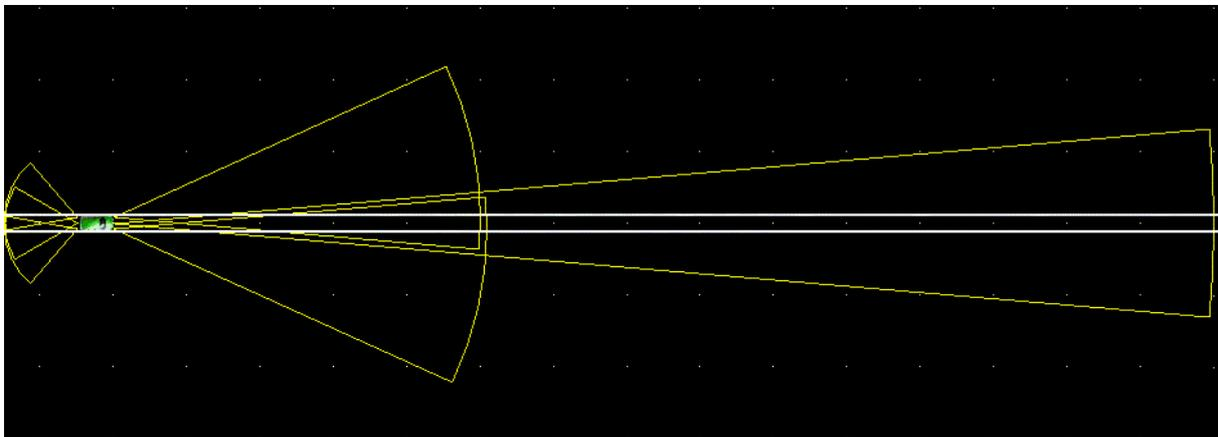
Figure 1: Example Radar Combination: 1xLRR(10°,150m), 2xMRR(30°,50m), 3xSRR(60°,10m)
