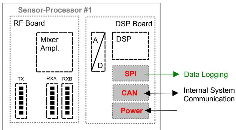
Figure 3: Bloc Diagram of the UMRR Radar Sensor
