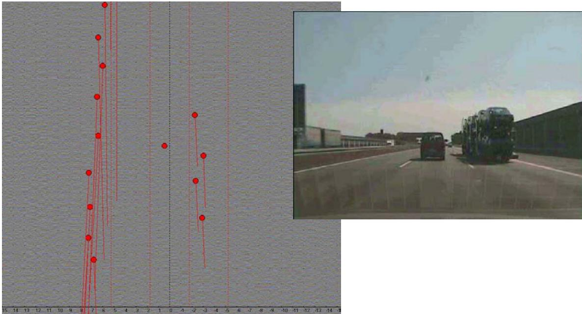
Figure 4: Autobahn scenario: detected radar targets and photograph of the situation.
